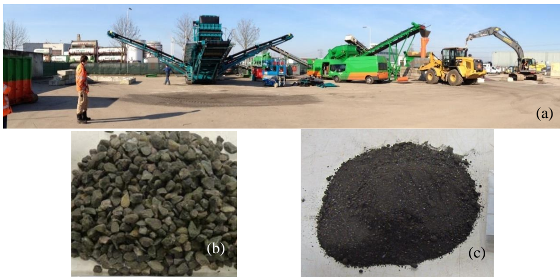
Figure 2. (a) the LE2AP decomposition process; (b) reclaimed aggregates, PA-stone; (c) reclaimed mortar sand
